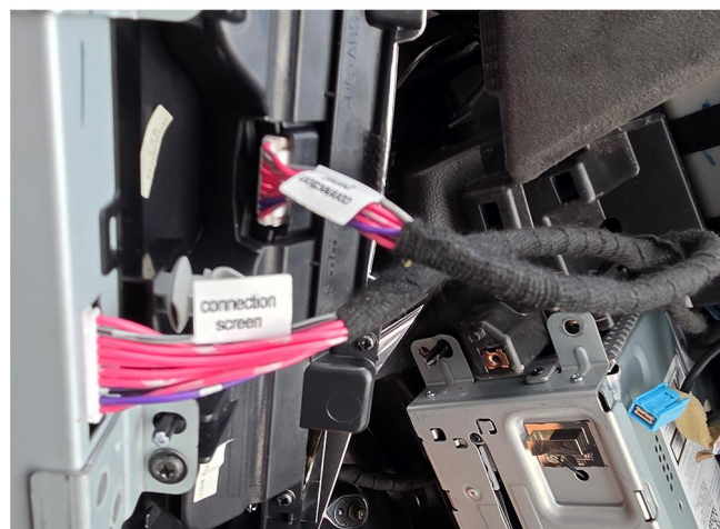
16. Connect the screen and button "Y" loom as shown:
