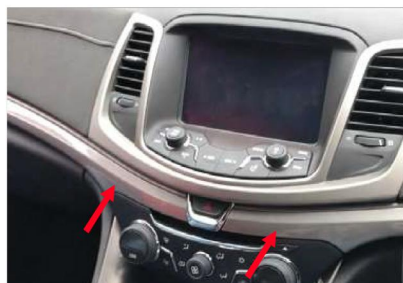
1. Remove the trim plate from the center console
