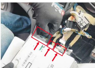
7. Unplug the main lines and video cable on the original head unit
