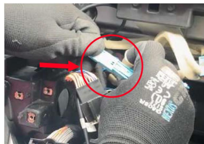
13. Dock the LVDS cable of CarPlay with video cable of the head unit
