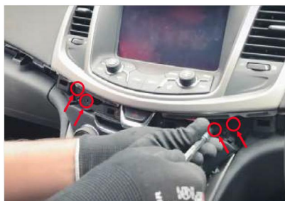
2. Unscrew the screws on the screen
