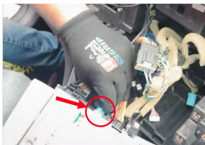
12. Connect the CarPlay LVDS cable to the original car head unit
