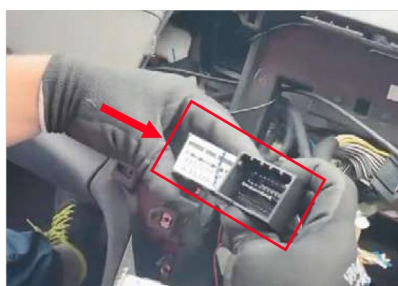
8. Connect the CarPlay main line with the original car main line
